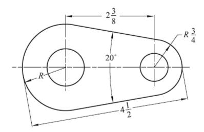
11) Determine angle A. The dimensions shown are in inches.
